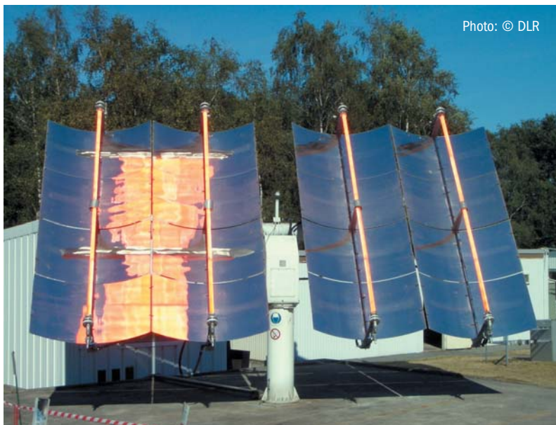
Pilot plant for the photochemical synthesis of fine chemicals
